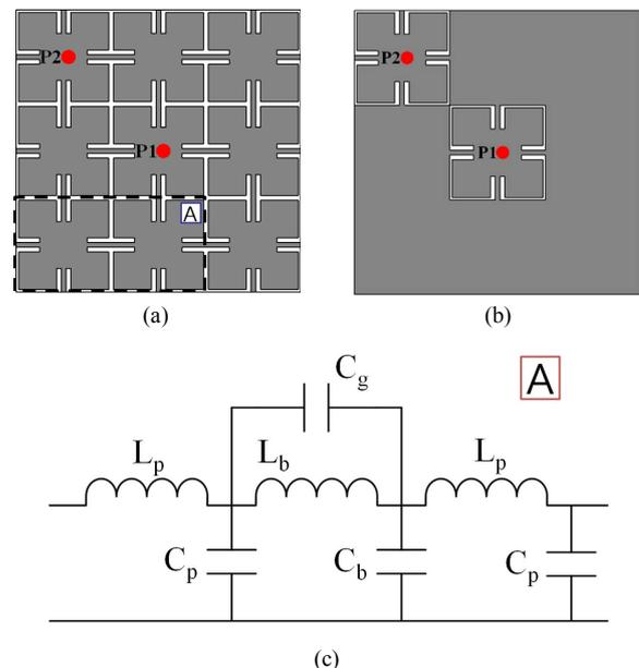
Fig. 1 Conventional EBG structure (a) Periodic EBG structure [5] (b) Localized EBG structure (c) Equivalent circuit model for the two connecting unit cells in Fig. 1(a) [5]
