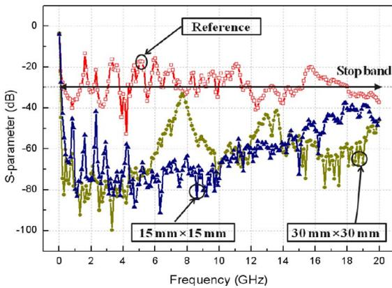
Fig. 5 The measured results of the proposed localized EBG structures
