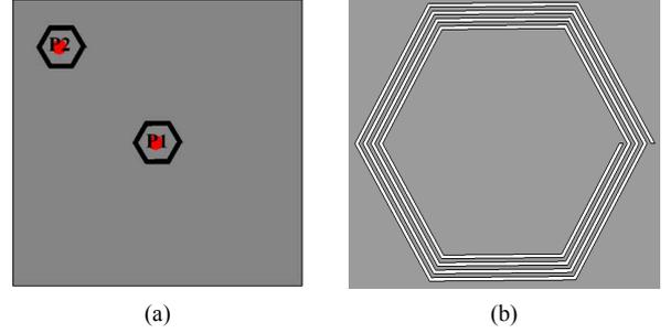
Fig. 2 Proposed spiral-shaped EBG Structure (a) The localized EBG structure (b) The proposed unit cell
