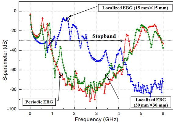
Fig. 4 Measured results of periodic and localized conventional EBG structures
