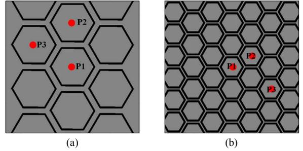
Fig. 3 Proposed periodic spiral-shaped EBG Structure (a) 30 mm×30 mm unit cell (b) 15 mm×15 mm unit cell
