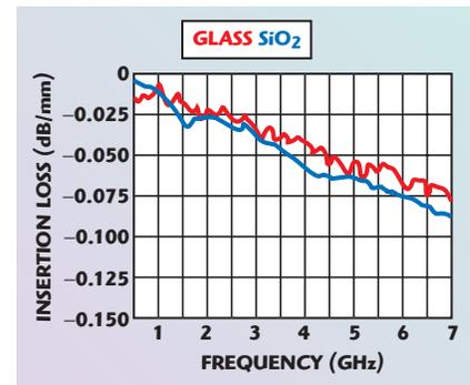
▲ Fig. 1 Insertion loss of coplanar transmission lines on 25  $\mu\text{m}$  thick oxide Si substrate and high quality glass substrate.
