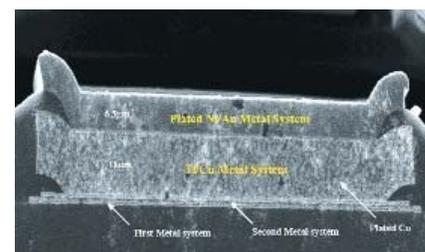
▲ Fig. 3 Cross-sectional view of a bonding pad.
