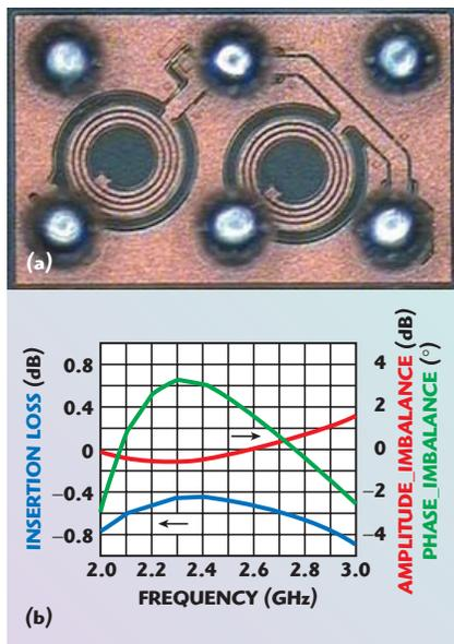
▲ Fig. 8 Balun for 2.4 GHz wireless LAN applications (a) and its measured results (b).
