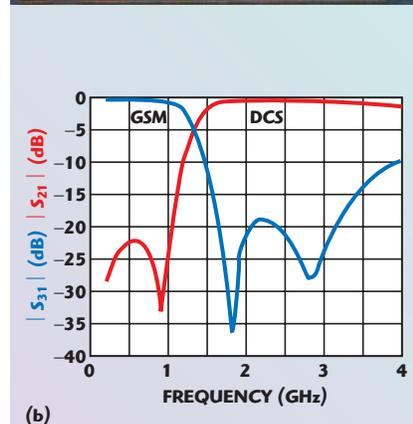
▲ Fig. 6 GSM/DCS diplexer (a) and its measured results (b).
