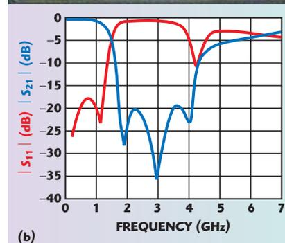
▲ Fig. 5 Wafer-level packaged low pass filter (a) and its measured results (b).
