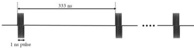
**Figure 1** Timing chart of the transmitted pulses
