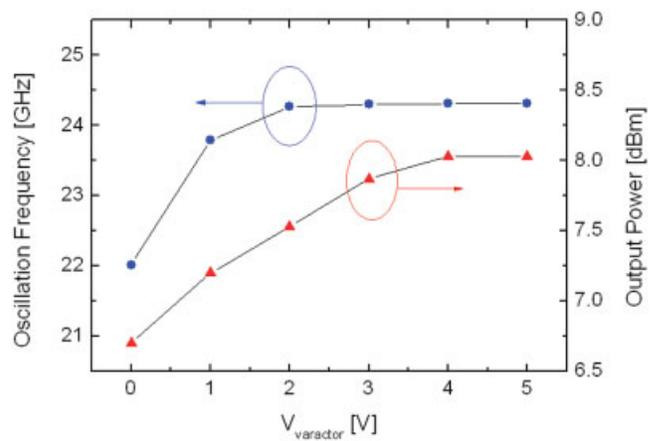
**Figure 5** CW-oscillation frequency and output power of the VCO with the varactor tuning voltage. [Color figure can be viewed in the online issue, which is available at [www.interscience.wiley.com](http://www.interscience.wiley.com)]
