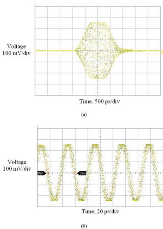
**Figure 6** A 24 GHz pulse waveform (The signal amplitude was intentionally attenuated to show the entire waveform in an oscilloscope window. The real amplitude is approximately 1.4 Vpp). [Color figure can be viewed in the online issue, which is available at [www.interscience.wiley.com](http://www.interscience.wiley.com)]
