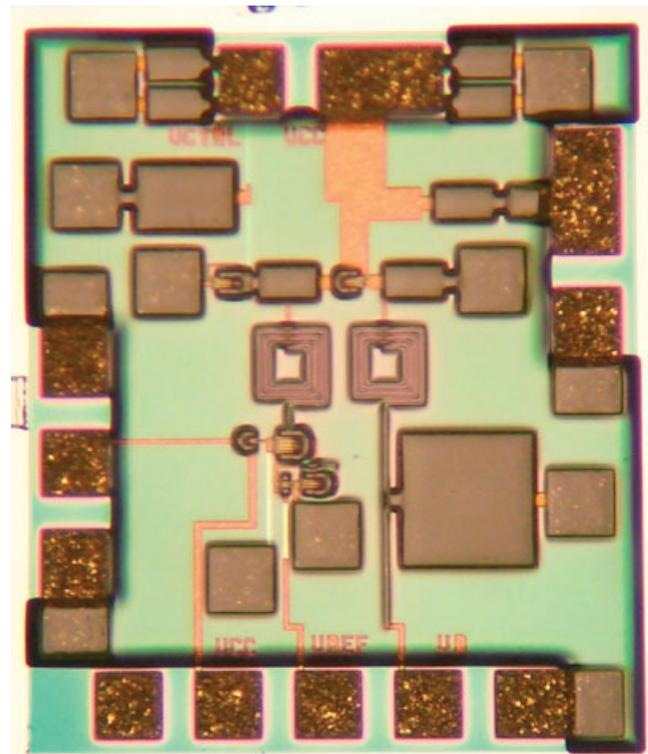
**Figure 3** Photograph of the fabricated pulse VCO. [Color figure can be viewed in the online issue, which is available at [www.interscience.wiley.com](http://www.interscience.wiley.com)]
