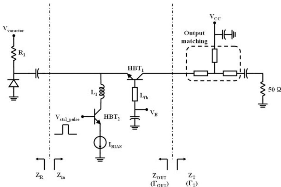
**Figure 2** Schematic diagram of the pulse VCO
