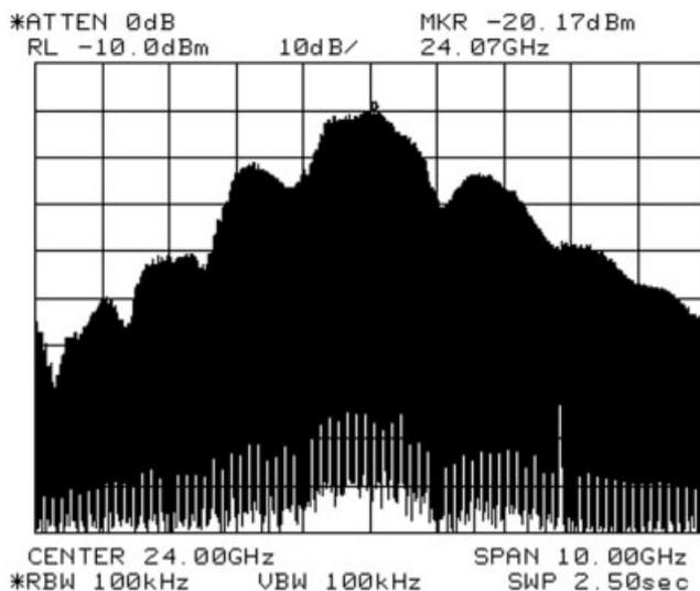
**Figure 7** Output spectrum of the pulse oscillator in pulse mode
